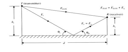
$E_{TOT} = E_{LOS} + E_{g}$  *Let*  $E_{0}$  is the free space E-field (V/m) at a reference distance  $d_{0}$  from the transmitter, then for  $d > d_{0}$
